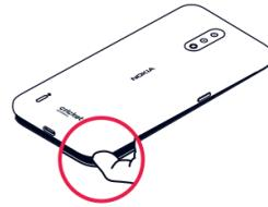
1. With the phone facing down, lace your fingernail in the seam between the back cover and the display, bend the back cover open, and remove it.
