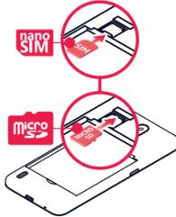
4. If applicable, hold the microSD card (sold separately) with metal contacts facing downward and the cut corner at the upper right. Slide the card into the microSD slot.
